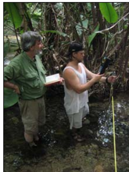
Duffy and French Measure the Stream Flow of the Picota with a Rickly Flow Tracker
